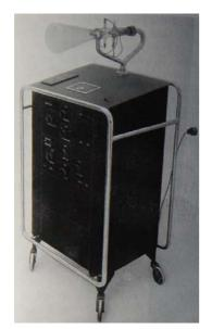
The first commercially built European Cathode - Ray Oscilloscope was developed in the German Manfred von Ardenne Laboratory at Berlin - Lichterfelde and manufactured from early 1932 at the small Swiss company Dipol AG, Arbon (Lake Konstanz), The power supply, the sweep generator as well as an optional vertical deflection amplifier were housed in the movable compartment. The Cathode Ray Tube built by Leybold und von Ardenne, Köln was mounted on a stand at the top of the compartment.
